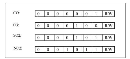
The R/W bit is also used as a common data bit. When reading/writing, use 1 or 0 perform 'OR' operation with original data (read as 1, write as 0). See the figure below for details.
